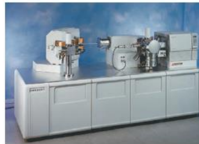
A double-focusing mass spectrometer. This one is combined with a gas chromatograph to use as a GC-MS. The gas chromatograph separates a mixture into its components and injects the purified components into the ion source of the mass spectrometer.
